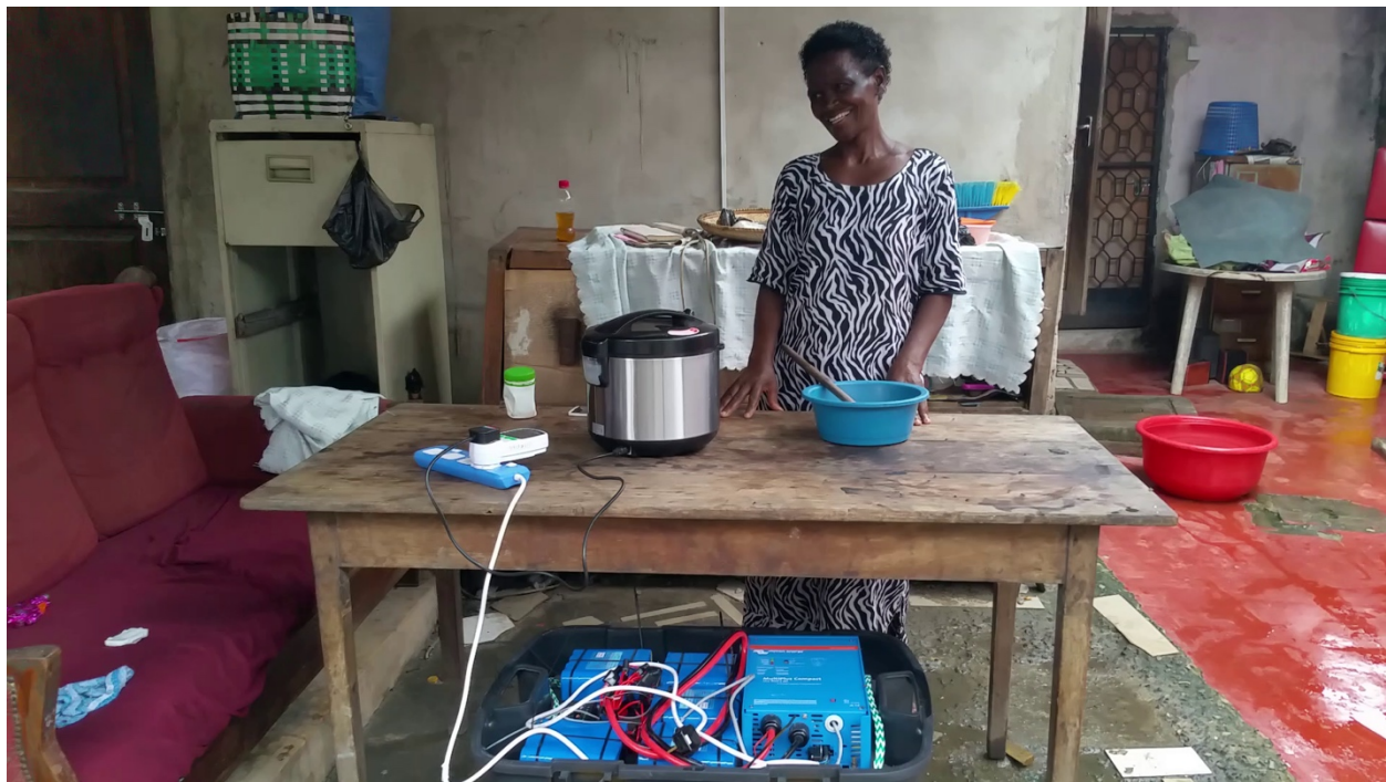
Figure 9: 'Under-the-table' mode (with lid off for the photo), allowing the cook to use the prototype as if the appliances were connected to the grid.
