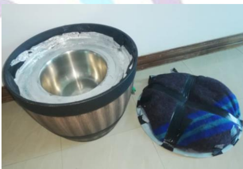
Image 21: Water heater with thick blanket taped to the underside of the lid
