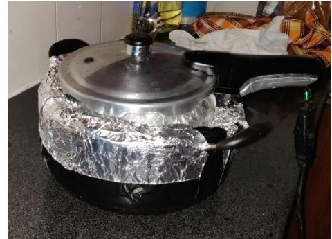
Image 20: Pressure cooker prototype in extra insulation
