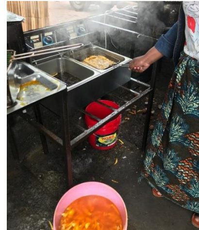
Image 18: Electric fryers are one of the only electrical devices available for chips
