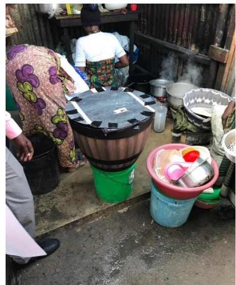
Image 3: Case study rice/bean vendor using solar water heater alongside their usual charcoal stoves, Sahara Market
