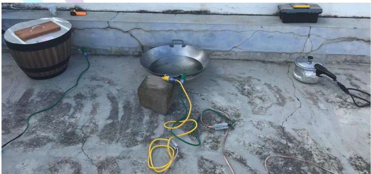
Image 6: The three prototypes (from left to right: water heater, wok and pressure cooker)
