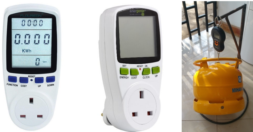
Figure 2: a) (left) Plug-in energy meters and b) hanging balance used to measure the total energy consumption of each heating event.
