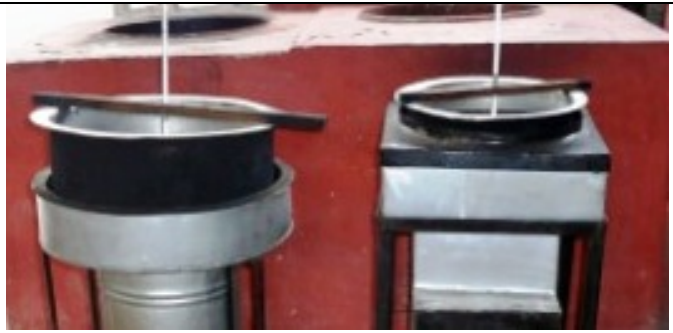
Figure 11: M&R and ENVOTEC stoves showing the difference in skirt height/diameter ratio
