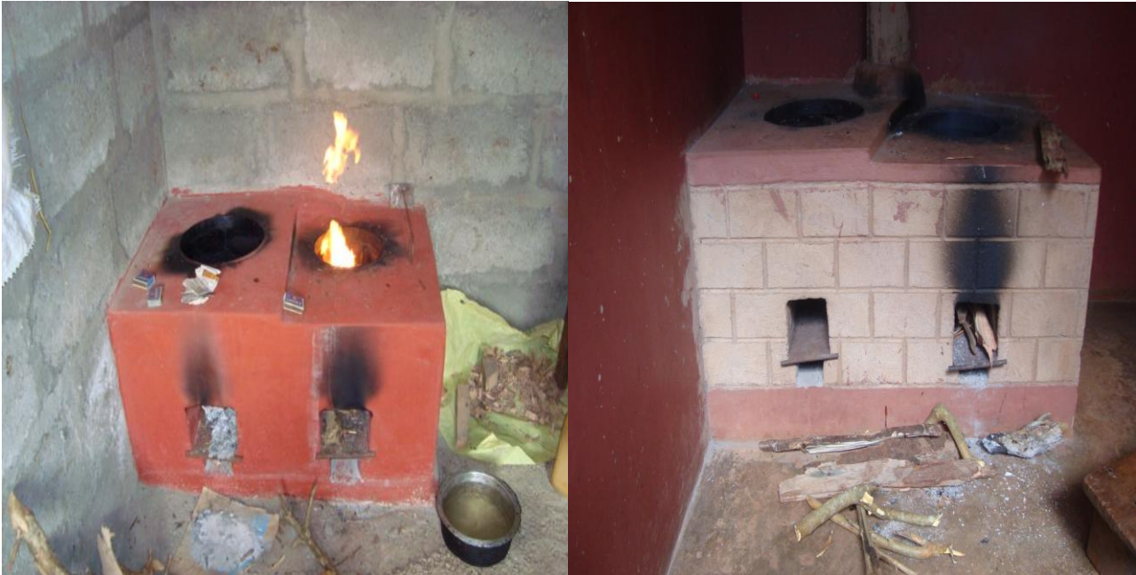
Figure b: Showing two pictures of Okoa number 1 stoves with two pot guards each.
