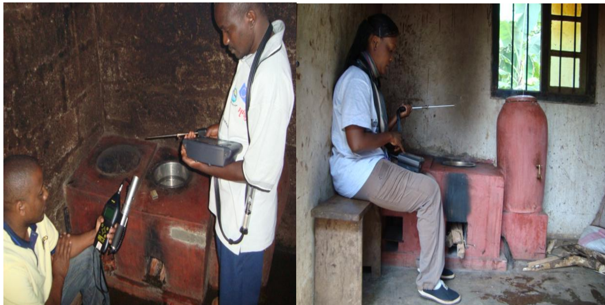
Figure 2: Air contaminants measurement using Combustion Gas Analyzer and Microdust pro devices.
