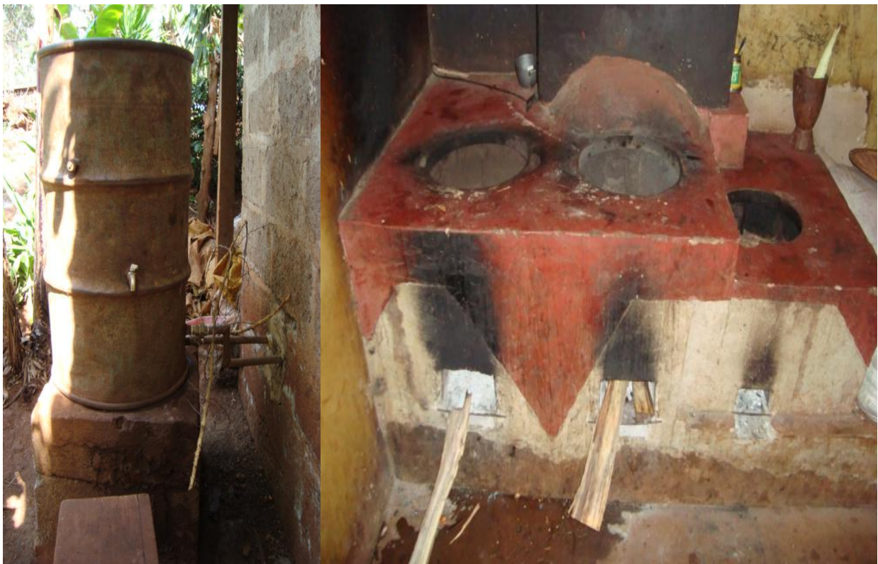
Figure g: Shows modified Okoa number 2 stove having three pot guards with a capacity of boiling water in a tank of 120 liters placed outside the kitchen.
