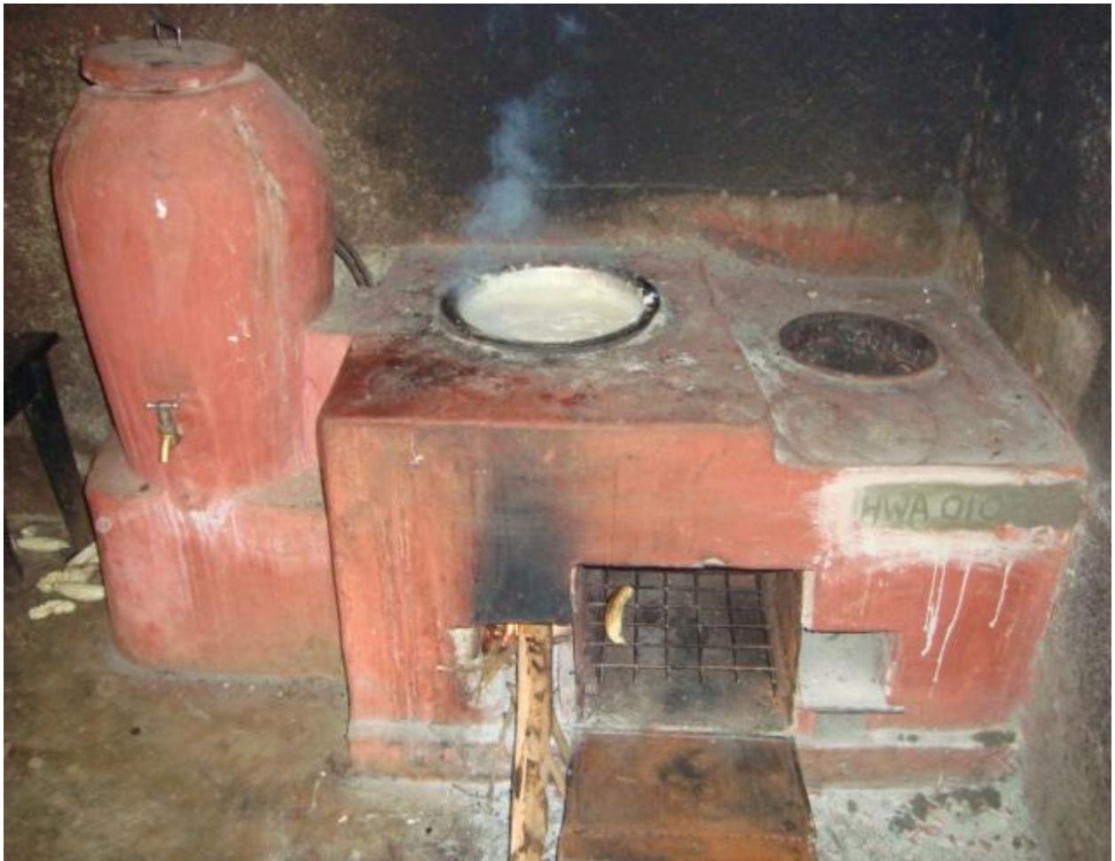
Figure d: Okoa stove number 3 having two pot guards, oven and water boiler pot with water tap.
