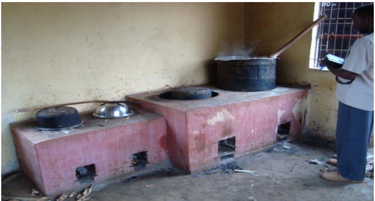
Figure e: Two in one Okoa number 1 stove, with four pot guards mostly found used in the Institutions like schools.
