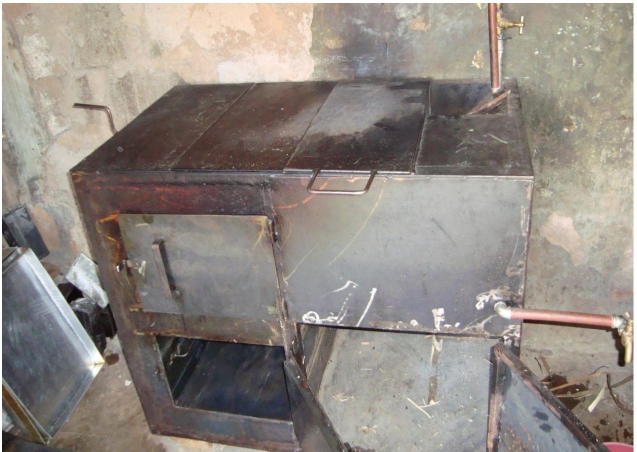
Figure h: Shows improved wood stove with chimney (presented by 3 pictures above) having four hot plates at the top for cooking, wood storage chamber, two bakery units and a water boiler chamber with a capacity of 20 liters.
