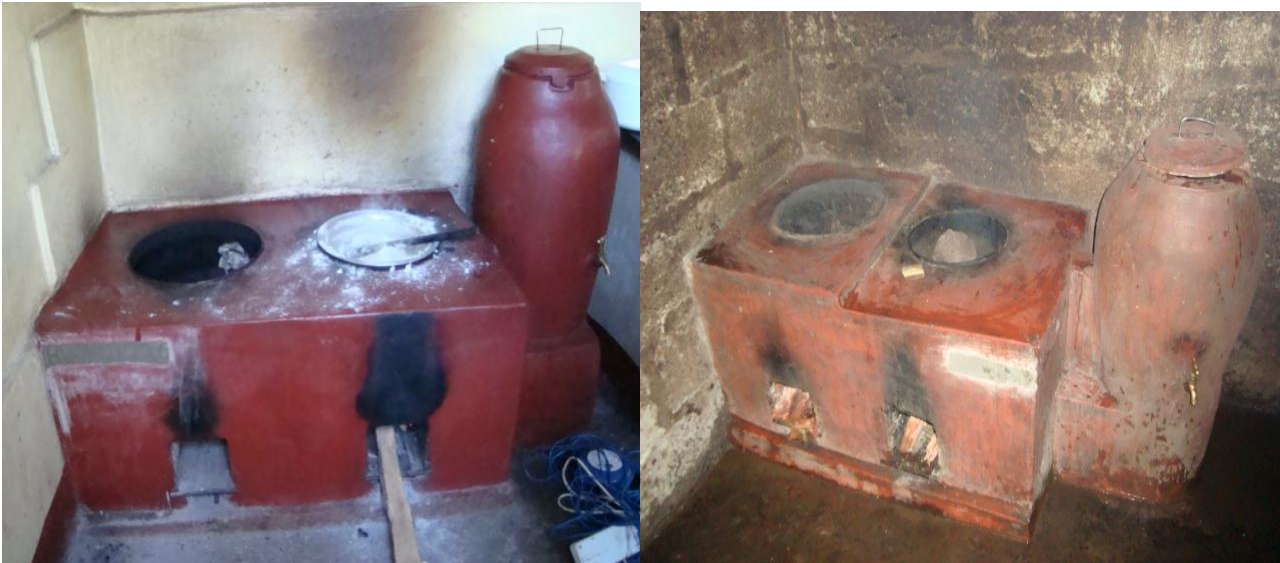
Figure c: Shows two pictures of Okoa number 2 stoves each having two pot guards and one water boiler pot with tap used in Hai and Rombo districts.
