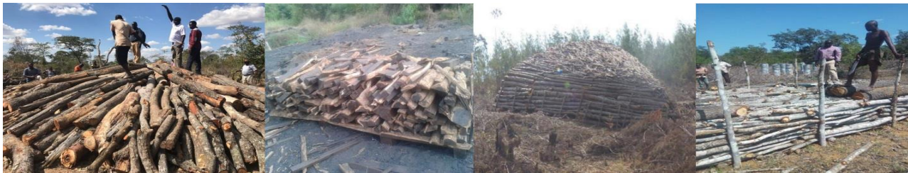
Figure 2: Common arrangement of logs in traditional kilns in Tanzania
